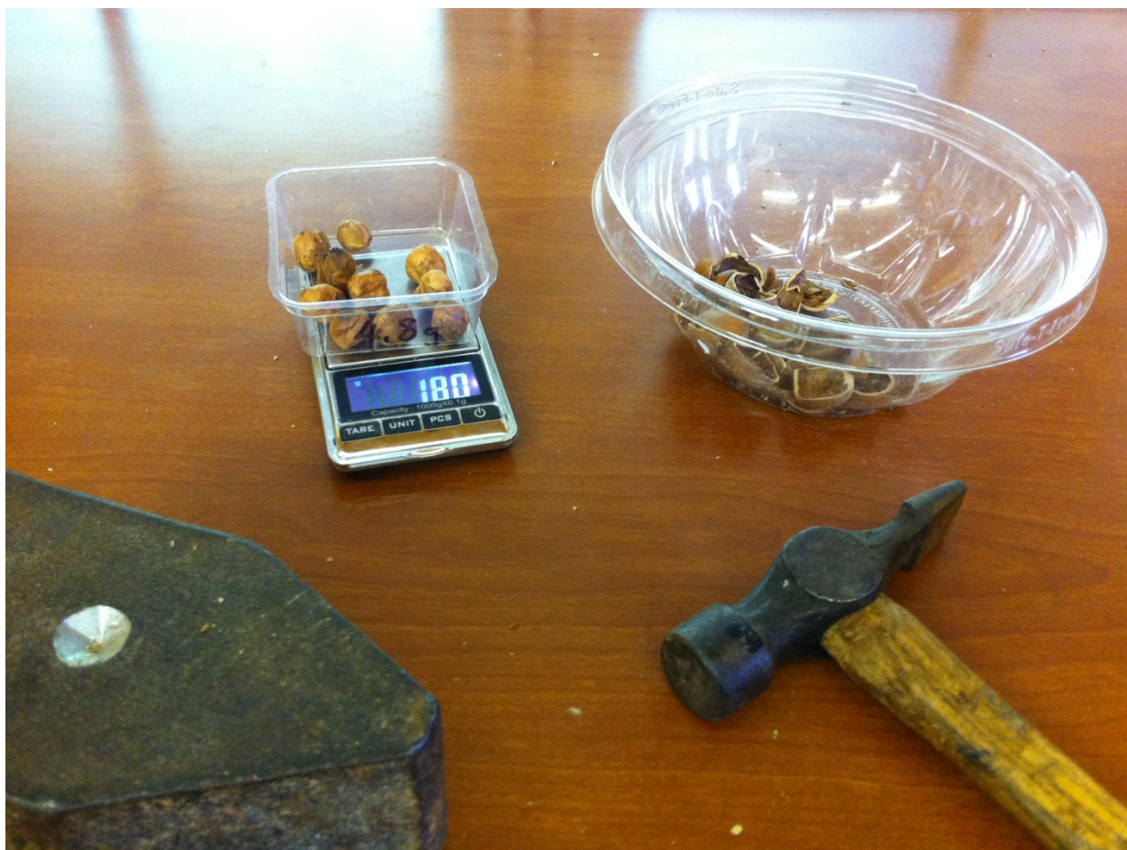
Figure C. Measuring the kernel yield of a 10 nut sub-sample.
